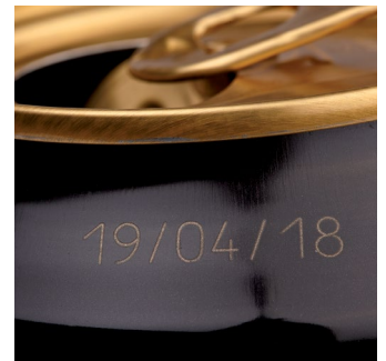
Color change of best before date of black anodized aluminum
