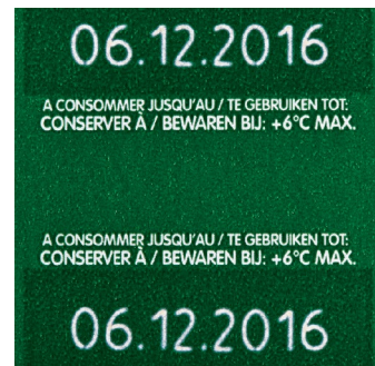
Expiration code Color removal on green foil
